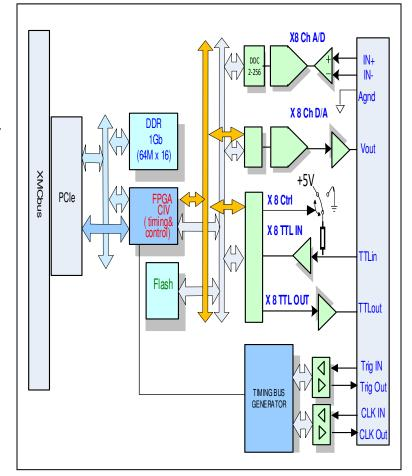
The XMC-MFIO-8 Simultaneously sampled A/D offers a mix of up to 8 Differential analog input channels at 8.192VP-P Fully Differential. All channel features handle analog input with a differential configuration for a rate up to 15Msps. The acquisition can be started by the host or by an on-board sequencer that uses a channel list to specify which channel to acquire. Each Channel has its own DDC that can be programmed independently for a decimation range from 2 to 256 programable in steps of 1.
